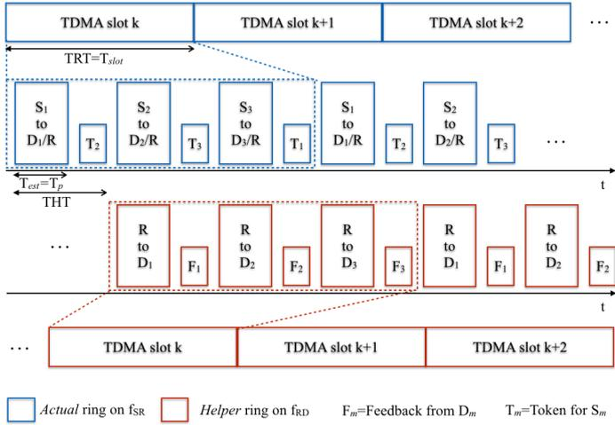
Fig. 2. Events timeline (frame structure) for proposed DRBF-TDMA system ( $M = 3$ ).
