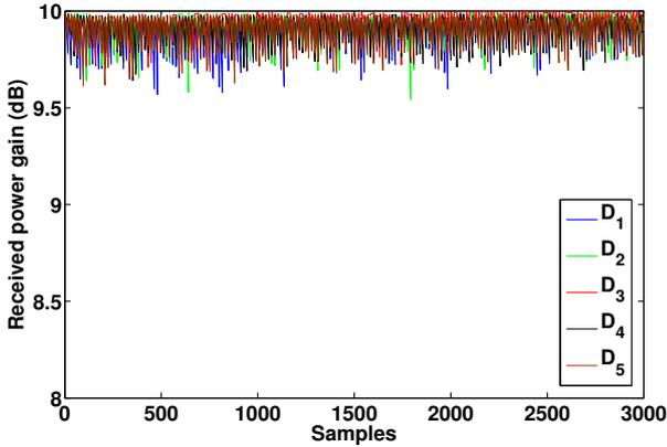
Fig. 7. Received power gains due to AF-DRBF.
