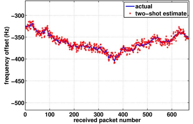
Fig. 4. Two-shot frequency offset estimation at relay  $R_1$ .
