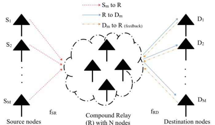
Fig. 1. Proposed DRBF-TDMA system architecture.
