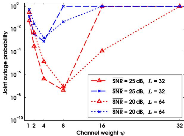
Figure 4. Additional impact of transmit power and bandwidth (number of usable sub-channels) for  $I_{out} = 128$  bit (red) and  $I_{out} = 256$  bit (blue)
