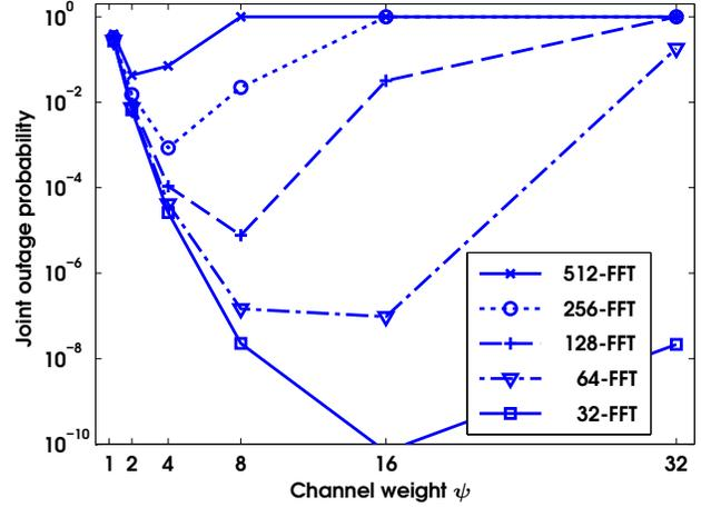
Figure 3. Additional impact of bandwidth (FFT size) on joint outage probability ( $\bar{\gamma} = 20 \text{ dB}$ ,  $I_{out} = 256$  bit)
