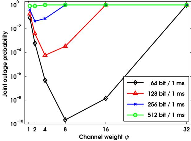
Figure 2. Dependence of joint outage probability on channel weight factor
