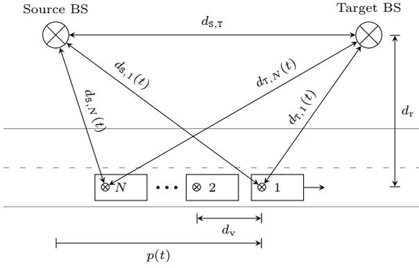
Figure 2. Geometric view of the considered platooning scenario.
