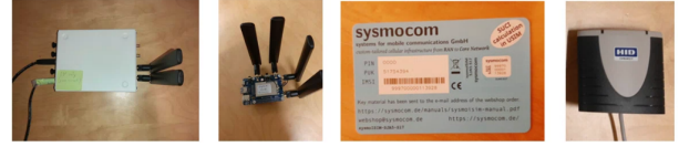
Fig. 3. From left to right: the USRP B210 SDR, the Quectel RF module, the SIM cards inserted at the Quectel module, and the SIM card reader to configure the cards. Our guide in [5] describes how to setup the testbed in Fig. 2 using this hardware and Ubuntu PCs.
