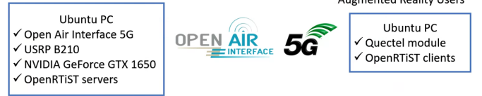
Fig. 2. A diagram of our open-source testbed. The clocks of the two Ubuntu PCs are synchronized by PTP to accurately measure the delays incurred in UL, DL, and at the edge.
