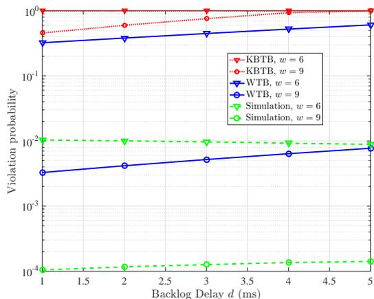
Fig. 16: Delay violation probability vs. backlog information delay  $d$  for a 3-hop network for different  $w$  with packet train arrival process ( $T = 5$ ),  $x_n = 33$ ,  $\rho = 25$ ,  $\sigma = 0$ , and SNR = 5 dB.
