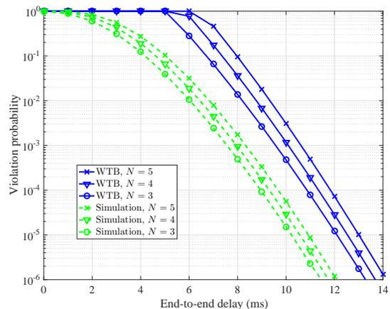
Fig. 14: Delay violation probability vs. end-to-end delay for different  $N$  with packet train arrival process ( $T = 5$ ),  $x_n = 100/N$ ,  $\rho = 25$ ,  $\sigma = 0$ , and  $\text{SNR} = 5$  dB.
