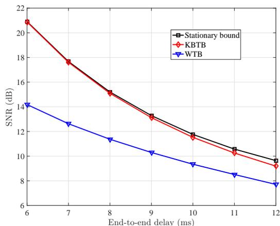
Fig. 9: SNR vs. end-to-end delay for a delay violation probability requirement of  $10^{-9}$  for a 2-hop network with packet train arrival process ( $T = 5$ ),  $x_n = 100$ ,  $\rho = 25$  and  $\sigma = 0$ .
