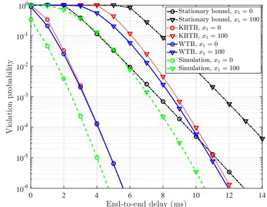
Fig. 6: Delay violation probability vs. end-to-end delay for a single link with burst arrival ( $T = 1$ ), SNR = 5 dB,  $\rho = 0$ , and  $\sigma = 25$ .
