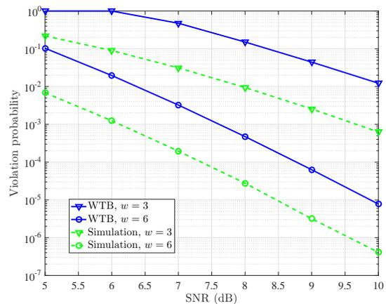
Fig. 10: Delay violation probability vs. average SNR for a 2-hop network for different target delays  $w$  with packet train arrival process ( $T = 5$ ),  $x_n = 50$ ,  $\rho = 25$ , and  $\sigma = 0$ .
