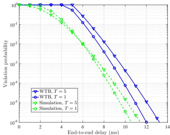
Fig. 12: Delay violation probability vs. end-to-end delay for a 3-hop network for different  $T$ ,  $x_n = 33$ ,  $\rho = 25$ ,  $\sigma = 0$ , and  $\text{SNR} = 5$  dB.
