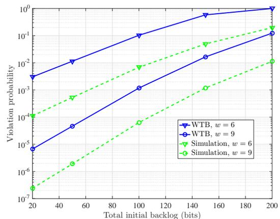
Fig. 11: Backlog violation probability vs. total initial backlog for a 2-hop network for different delays  $w$  with packet train arrival process ( $T = 5$ ),  $\rho = 25$ ,  $\sigma = 0$ , and SNR = 5 dB.
