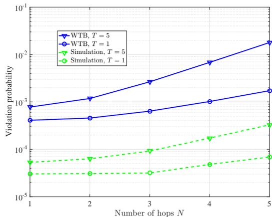
Fig. 13: Delay violation probability vs.  $N$  for different  $T$ ,  $w = 9$ ,  $x_n = 100/N$ ,  $\rho = 25$ ,  $\sigma = 0$ , and  $\text{SNR} = 5$  dB.
