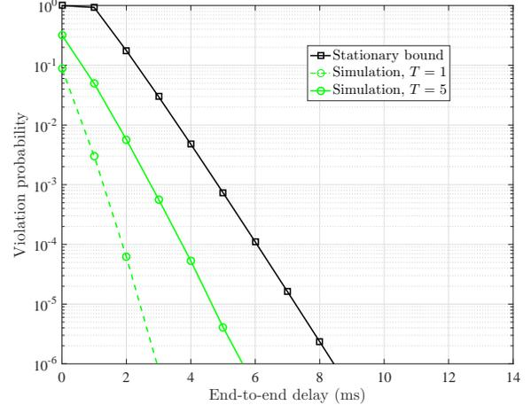
Fig. 3: Delay violation probability vs. end-to-end delay for a single link with SNR = 5 dB,  $x_1 = 0$ ,  $\rho = 20$ ,  $\sigma = 0$ .
