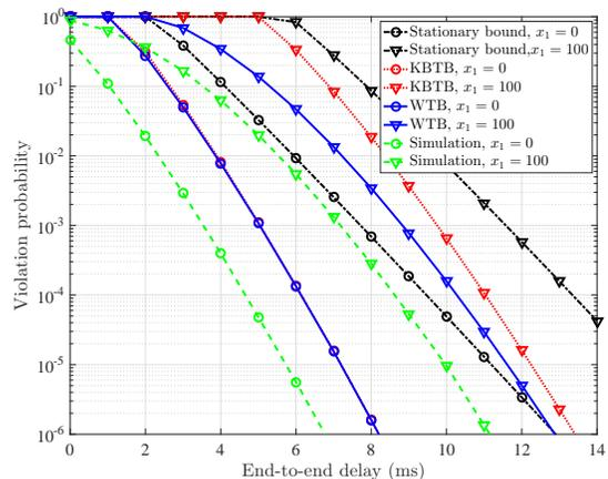
Fig. 7: Delay violation probability vs. end-to-end delay for a single link with the packet train arrival process ( $T = 5$ ), SNR = 5 dB,  $x_1 = 100$ ,  $\rho = 25$  and  $\sigma = 0$ .
