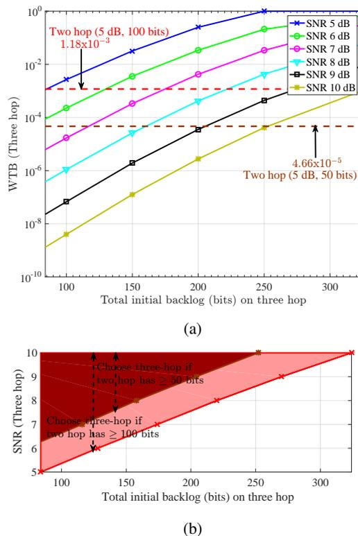
Fig. 17: (a) WTB for the 3-hop route (solid lines) versus the total initial backlog for different SNRs and  $w = 9$  ms; WTB for the 2-hop route (dotted lines) with SNR = 5 dB, and total initial backlogs 50 bits (bottom) and 100 bits (top). (b) Decision region for choosing 3-hop route over 2-hop route with different total initial backlogs.
