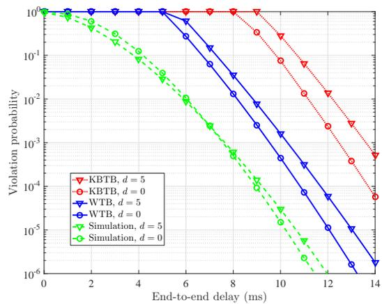
Fig. 15: Delay violation probability vs. end-to-end delay for a 3-hop network for different  $d$  with packet train arrival process ( $T = 5$ ),  $x_n = 33$ ,  $\rho = 25$ ,  $\sigma = 0$ , and  $\text{SNR} = 5$  dB.
