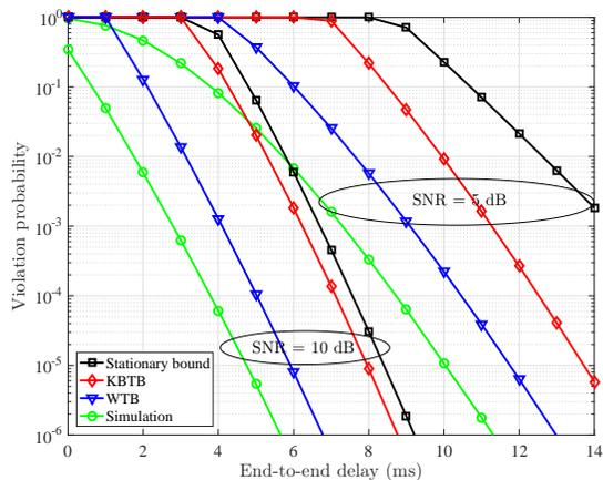
Fig. 8: Delay violation probability vs. end-to-end delay for a 2-hop network with the packet train arrival process ( $T = 5$ ),  $x_n = 100$ ,  $\rho = 25$  and  $\sigma = 0$ .
