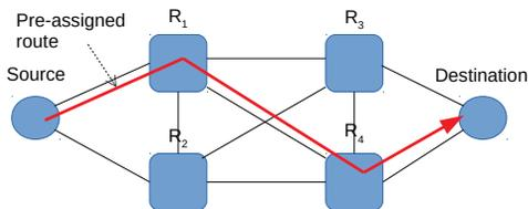
Fig. 4: Example of wireless mesh topology with a static route.
