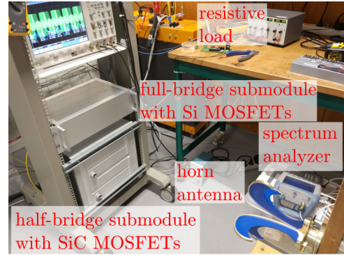
Fig. 3. Experimental setup of the submodules: full-bridge submodule with Si MOSFETs enclosed in an aluminum 19-inch rack, half-bridge submodule with SiC MOSFETs enclosed in an aluminum enclosure.
