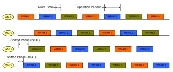
Figure 4. Phase-shifting DFH Operation
