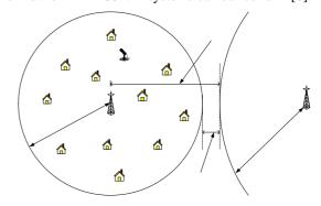
Figure 1. A Typical 802.22 WRAN Cell coexisting with DTV and Part 74
