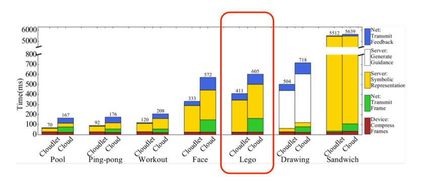
QoE determined by latencies  $t_{low}$ =600 ms,  $t_{up}$  = 2.7 s !
