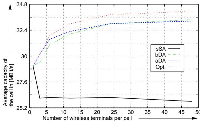
Figure 1. Capacity of the cell for a varying number of wireless terminals in the cell for the sSA, bDA, aDA and the optimal assignment in case of a transmit power per subcarrier of  $-7$  dBm
