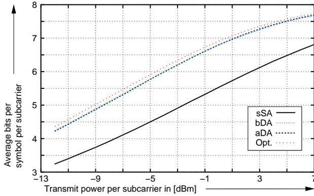
Figure 3. Average number of bits transmitted per subcarrier for the sSA, bDA, aDA and the optimal assignment for a varying transmit power in the case of 48 terminals present in the cell
