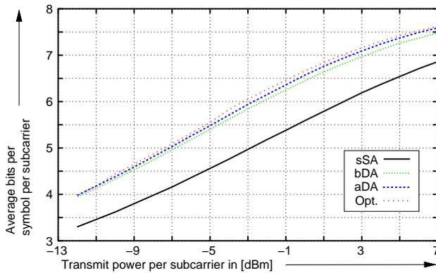
Figure 4. Average number of bits transmitted per subcarrier for the sSA, bDA, aDA and the optimal assignment for a varying transmit power in the case of six terminals present in the cell
