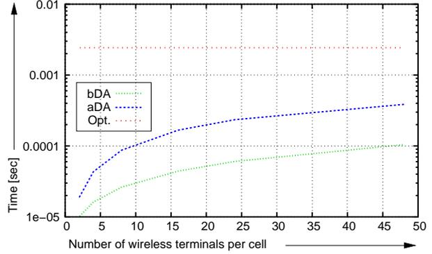
Figure 5. Logarithmic plot of average run time values for the bDA, aDA and the optimal assignment with a fixed number of subcarriers ( $S = 48$ ) and an increasing number of wireless terminals in the cell
