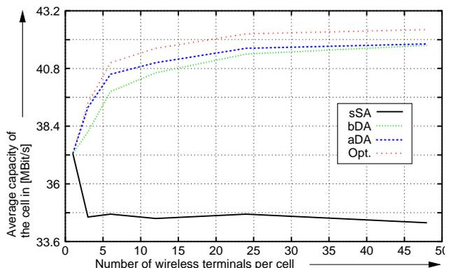
Figure 2. Capacity of the cell for a varying number of wireless terminals in the cell for the sSA, bDA, aDA and the optimal assignment in case of a transmit power per subcarrier of 0 dBm
